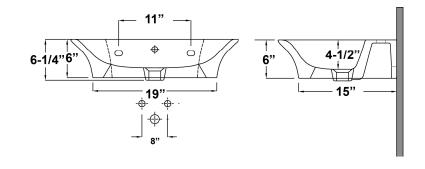
Dimensions of fixture are nominal and may vary within the range of tolerances established by ASME Standard A112.19.2.2018 Dimensions and specifications subject to change without notice.
